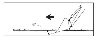
Use a slight bucket angle, travel forward, and hold the lift control forward to start the cut. Make a short, angle cut approximately 6" deep and break-out cleanly.
